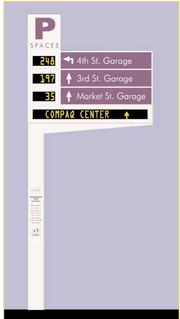
Proposed design for the Department of Transportation's Parking Guidance System. The system will inform motorists of parking locations and real-time space availability using electronic message signs located at Downtown gateways and intermediary points closer to parking facilities.
