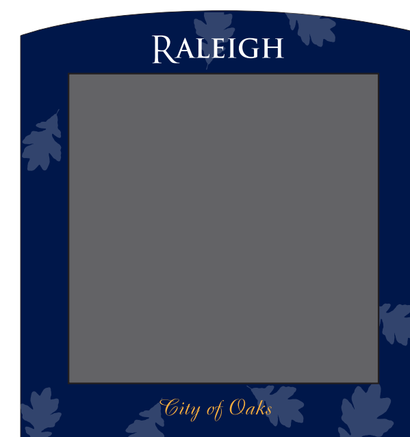
Sign Type M, Replacement Map Panel Surface mounted to end panel of existing newspaper racks. Overall fiberglass embedded graphic panel 44.5 x 47 inches with arched top.
