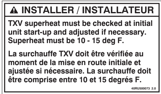
Fig. 21 - Label, TXV Adjustment
