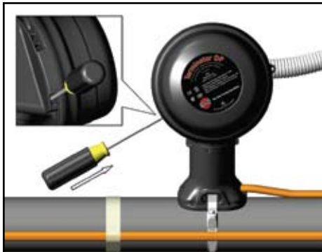
13. Install junction box lid and twist hand tight. Insert screwdriver into ratchet slots located on side of junction box base.
