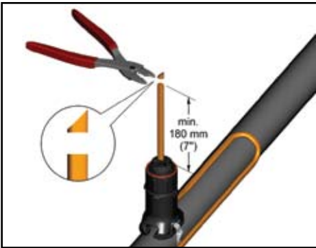
6. Cut off end of cable.
